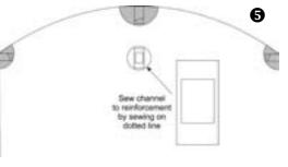
sail with a small zig-zag stitch. See Diagram 4. Construct the channel by centering the  $^7/8$ " x 1%" Dacron rectangle on the 1" x 1" Dacron rectangle. The short ends of each face top and bottom. Sew the smaller rectangle to the larger by sewing along ONLY the top and bottom edges with a straight stitch. Sew this assembly, with the smaller rectangle facing up, in the center of the
